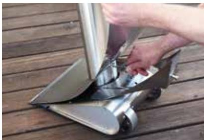
3. Tilt the sail and the tube slightly forwards so that the rod of the ash grid rises out of its holder for about 10 cm. Then turn the rod by 90° so that the ash drops into the pan.
