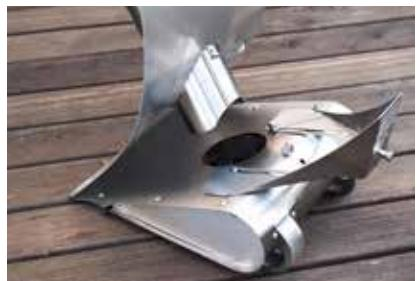
4. You can now remove the fire column with the heat shield from the ash pan.
