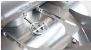
2. Then, close the protective cover and do not open it until the Feuersegel® has cooled down.
